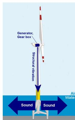
Fig. 8: Schematic representation of the entry of machine noise into the water [38]
