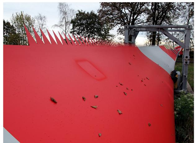
Fig. 5: Trailing edge serrations for mitigating noise emissions [6]
