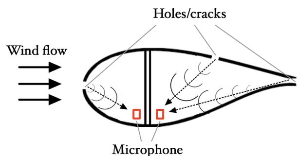
Fig. 1: Schematic illustration of acoustic measurement with passive damage detection (own illustration based on [13])
