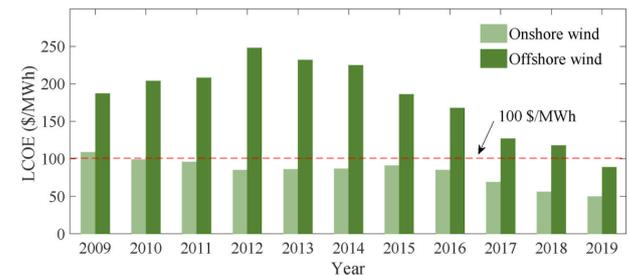
Fig. 1: Comparison of LCOE for onshore and OWTs between 2009 and 2019 [9]
