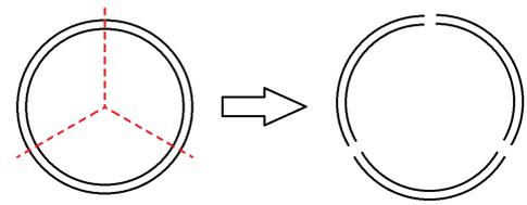
Fig. 4: Lengthways segmented tower segment (front view) [Source: Author]
