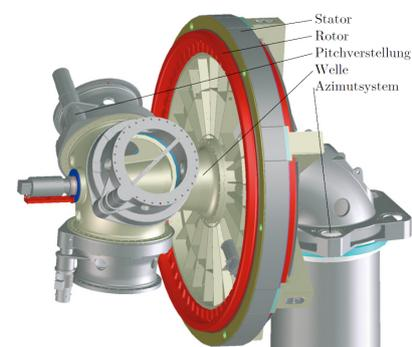
Fig. 3: Direct-drive turbine [6]
