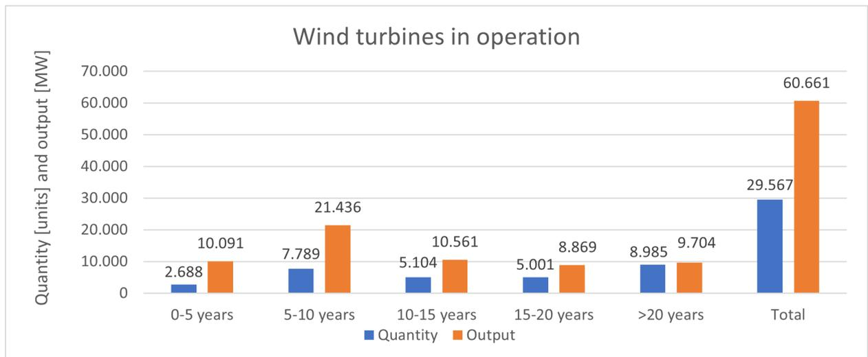
Fig. 1: Age structure of wind turbines in Germany (status 08.12.2023). Own illustration based on [3].
