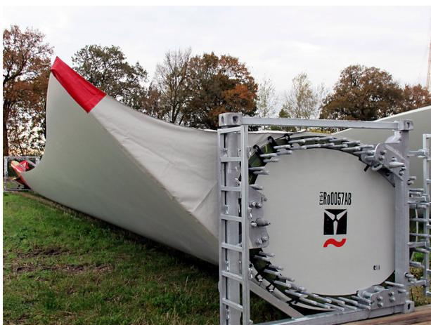
Fig. 2: Segmented rotor blade of an Enercon E115 with mechanical joints [6]
