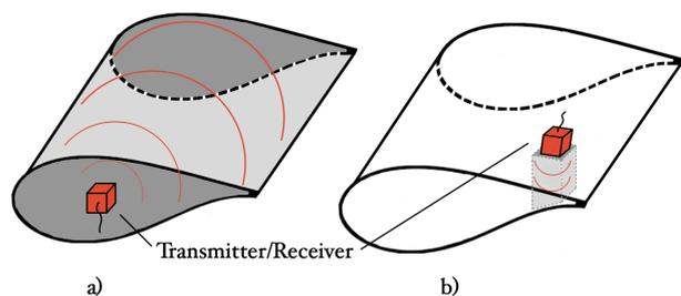
Fig. 3: The difference between a) ultrasonic guided wave measurement and b) conventional ultrasonic measurement
