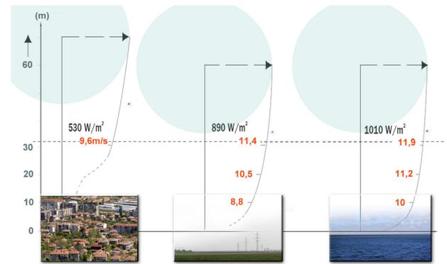
Fig. 1: Wind potential in different environments [12]
