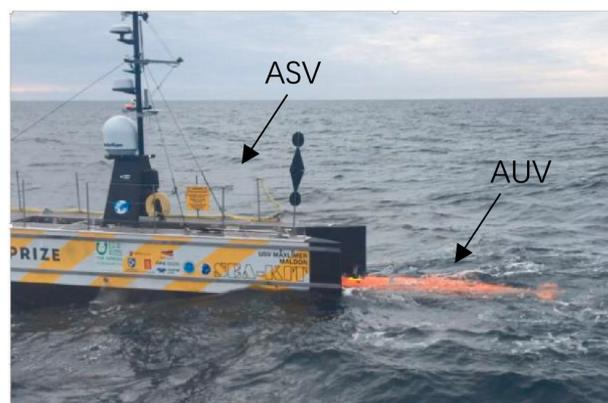
Fig. 6: Sea-kit Maxlimer ASVs recovering the HUGIN AUV [3]
