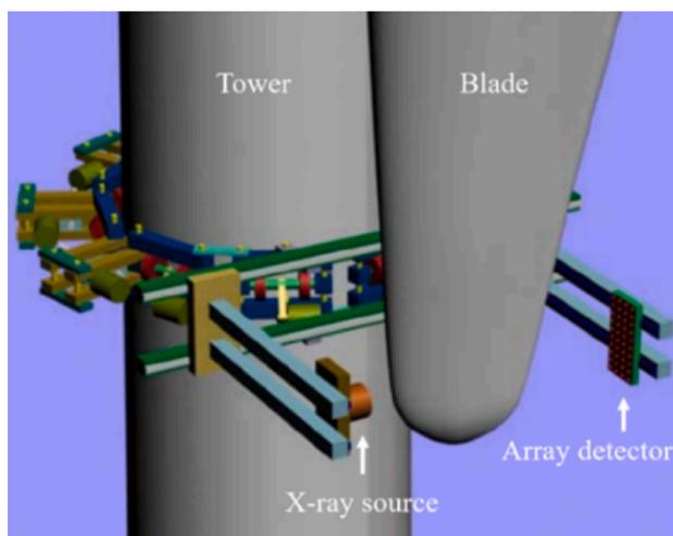
Fig. 3: Schematic illustration of a climbing robot for inspection of a OWT blade [2]
