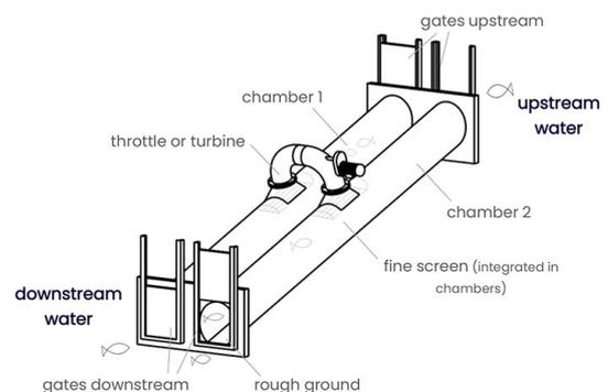
Fig. 3: Structure of the Fishcon fish pass [11].
