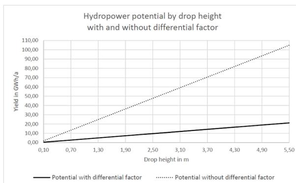
Fig. 1: Estimation of the total hydropower potential of wastewater treatment plant outlets in Germany
