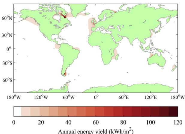
Fig. 1: The global theoretical tidal range energy resource calculated as annual energy yield ( $\text{kWh/m}^2$ ) per model grid cell ( $1/16^\circ \times 1/16^\circ$ ) [4], licensed under a Creative Commons Attribution (CC BY) license.
