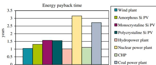
Fig. 4: Energy payback period for different energy sources [4]
