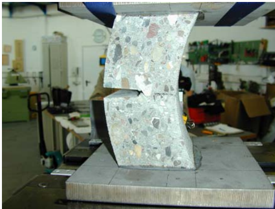
Fig. 7. New concrete pipe specimen, 9% ovality
