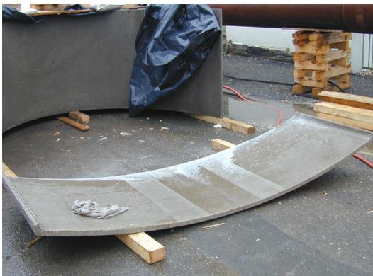
Figure 19. Polymeric concrete invert element
