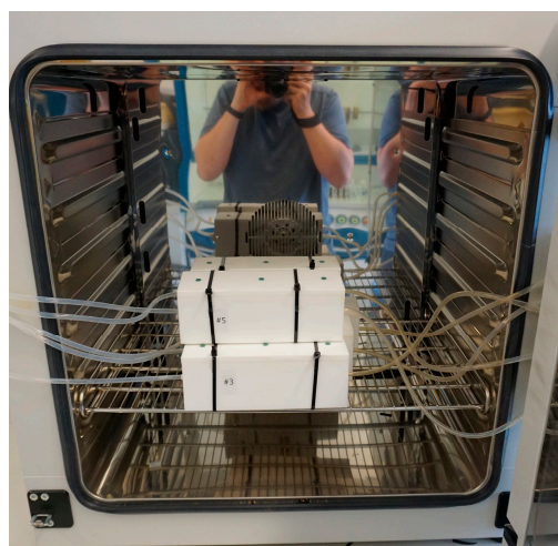
Figure 5. Sample chambers in laboratory oven. PTFE tubing attached to inlet (left) and outlet (right) of chambers.
