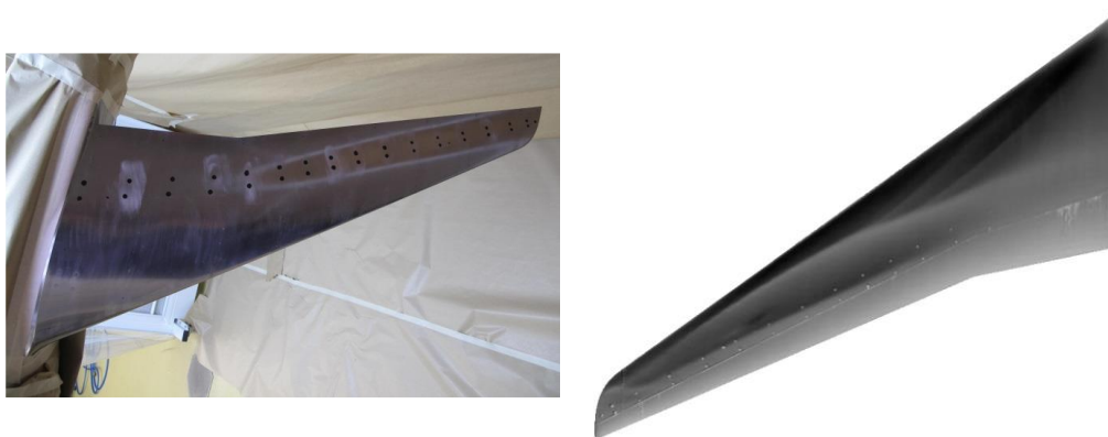
Figure 22. Left: PSP coating composed of PtTFPP as a sensor dye and PTMSP as binder on the lower side of a wing. Right: Pressure distribution on the upper side of wing model at test conditions Re = 25 \times 10^6 (Reynolds number), T = 296 K, angle of attack = 1^\circ . Luminescence lifetime data were converted to pressure coefficients and displayed [176]. Copyright © 2018 by the American Institute of Aeronautics and Astronautics, Inc.
