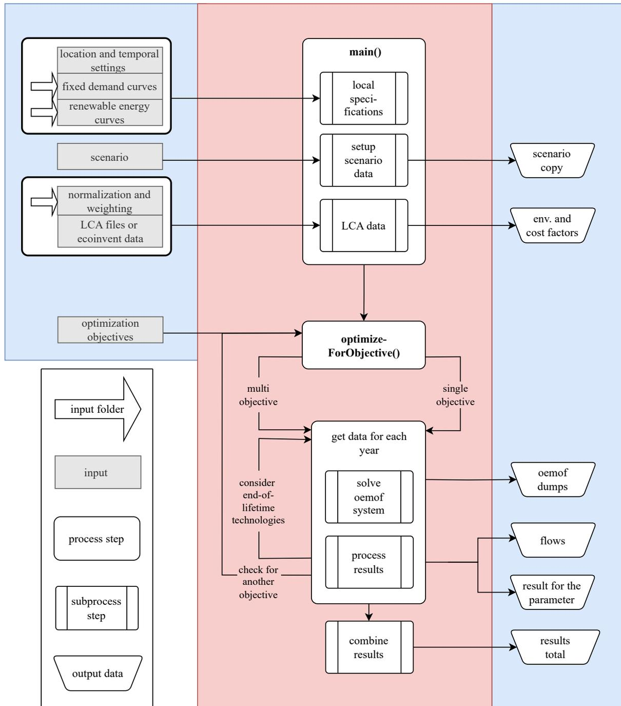
Figure 2.9.: Modeling workflow Life Cycle Assessment based Energy Decision (LAEND) Tool. The two main functions of the tool are printed in bold. Abbreviations: LCA = life cycle assessment, env. = environmental, oemof = Open Energy Modelling Framework. Own illustration based on [80, 81].
