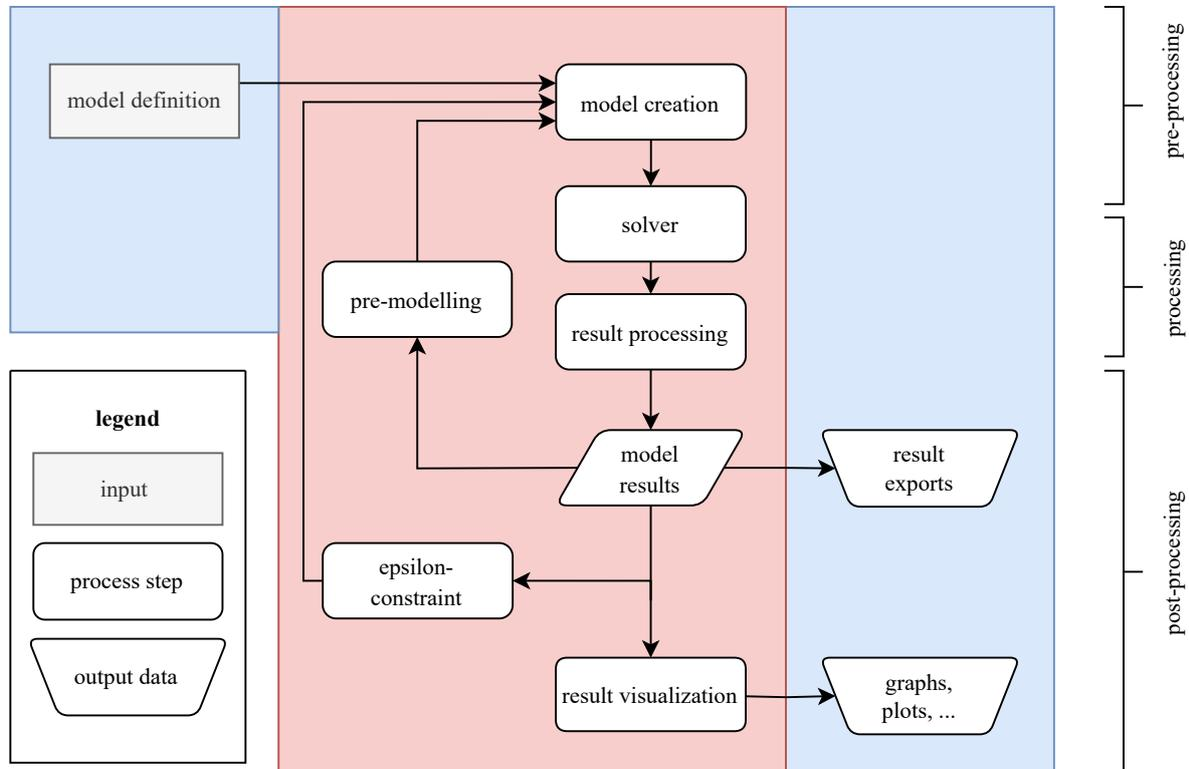
Figure 2.2.: Modeling workflow **SESMG**. Data represented as trapezoids (model results) can be accessed. Own illustration adapted from [32].
