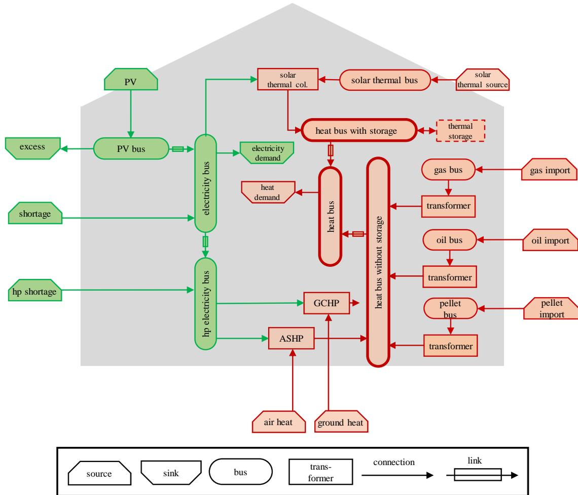
Figure 4.1.: Energy graph of the reference case. Containing all technologies from Table 3.3. Green represents electricity related components, red represents heat related components. Bold lines highlight the division of the heat bus into two buses. Abbreviation: PV = photovoltaic, solar thermal col. = solar thermal collector, hp = heat pump, ASHP = air source heat pump, GCHP = ground-coupled heat pump. Own illustration.
