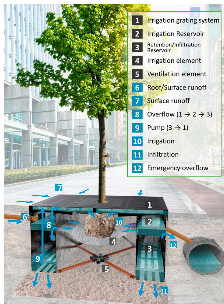
Figure 1. Overview of the stormwater tree pit system ALVEUS (water flow paths represented by blue arrows).
