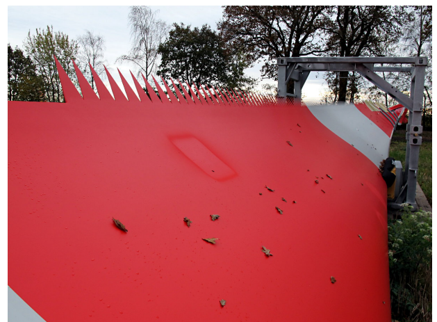
Fig. 5: Trailing edge serrations for mitigating noise emissions [6]
