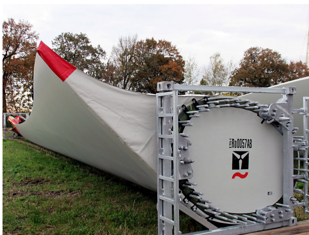
Fig. 2: Segmented rotor blade of an Enercon E115 with mechanical joints [6]
