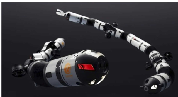
Fig. 5: The Eelume underwater robot was developed by NTNU and Equinor [1]
