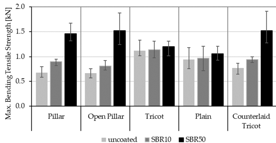
Figure 4. Maximum bending tensile strength of TRC samples under four-point bending test.
