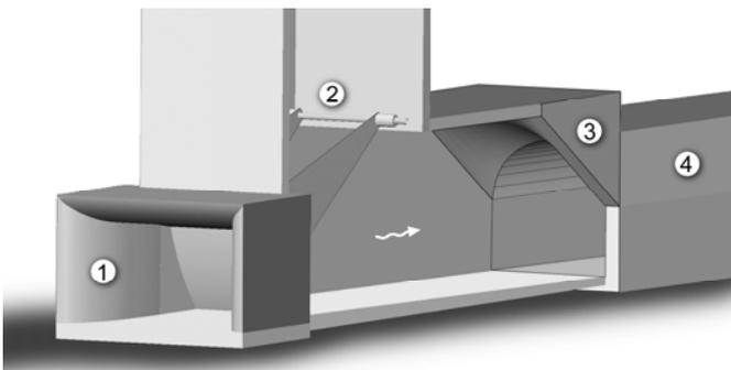
Figure 4: Bypass tunnel intake with (1) inlet trumpet, (2) tainter gate chamber, (3) shape distortion, (4) archway tunnel section.
