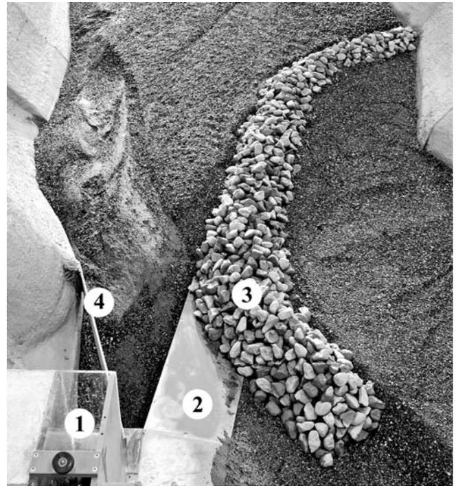
Figure 8: Upstream view from the (1) tunnel intake, (2) opening in the guiding structure and lowered part, respectively, (3) small rock fill dam as guiding structure, and (4) skimming wall.
