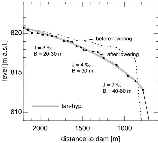
Figure 5: Longitudinal profile before and after the lowering test in prototype. The bed slope and the eroded channel width are denoted for different segments. The end profile follows a tangent hyperbolic function.
