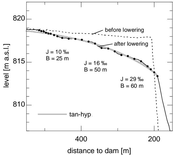
Figure 6: Longitudinal profile before and after the lowering test in the hydraulic model. The bed slope and the eroded channel width are denoted for different segments. The end profile follows a tangent hyperbolic function.
