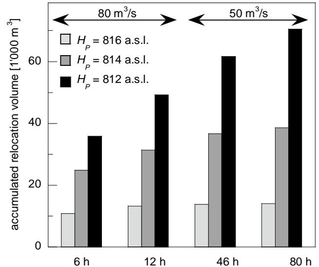
Figure 7: Accumulated relocation volume of sediment in the physical model at different times and for different lowered water levels  $H_p$ . The origin of the pivot point of the delta is at 818 m a.s.l. (Prototype dimensions).
