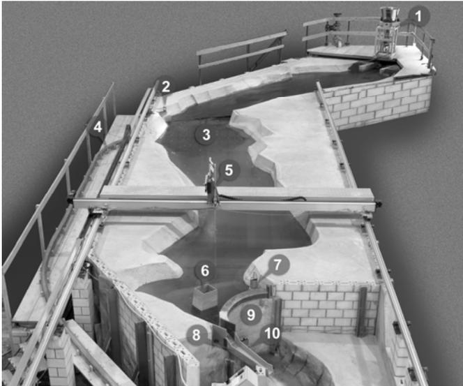
Figure 3: Hydraulic model with (1) sediment dosing machine, (2) bypass tunnel intake, (3) guiding structure, (4) bypass tunnel, (5) laser, (6) intake structure, (7) ultrasound device, (8) spillway, (9) dam and (10) bottom outlets.
