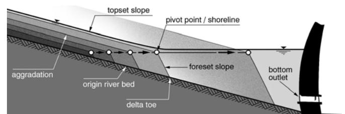
Figure 1: Schematic depiction of an aggradating coarse delta in a reservoir. In case of constant water level the pivot point moves ahead on a horizontal line whereas the topset slope is lifted up parallel to the origin river bed.
