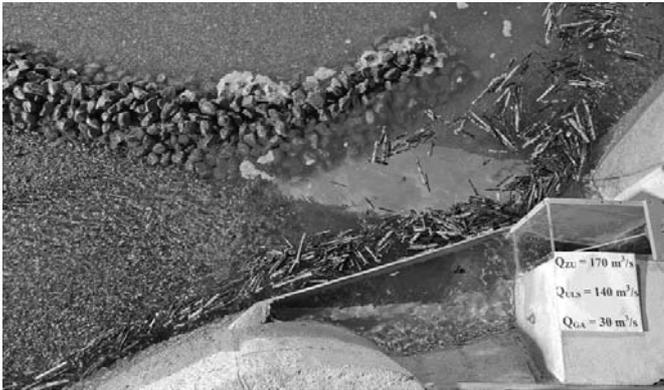
Figure 9: Driftwood model test with flow from left to right. Incoming discharge is  $170 \text{ m}^3/\text{s}$  ( $HQ_5$ ),  $140 \text{ m}^3/\text{s}$  are conducted through the bypass tunnel,  $30 \text{ m}^3/\text{s}$  pass by the tunnel intake along the skimming wall.
