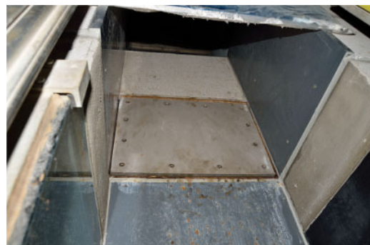
Figure 2. Plate microphone and plate vibration sensor in the test flume.
