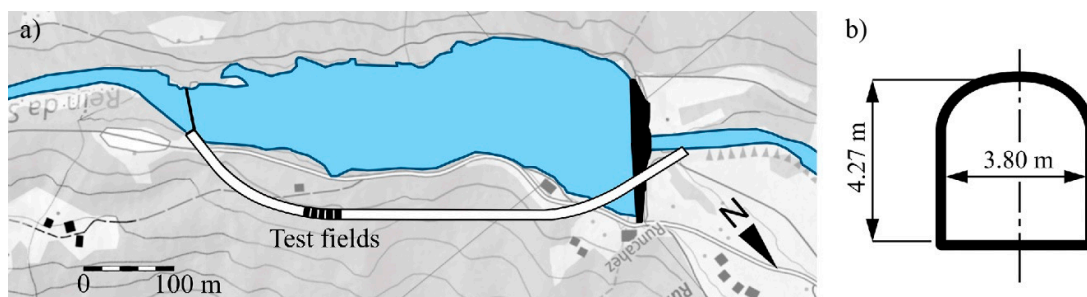
Figure 3. (a) Overview and (b) cross section of the Runcahez SBT (position 46^{\circ}40'45.0'' \text{ N } 8^{\circ}58'05.7'' \text{ E} ; adapted from [18]).
