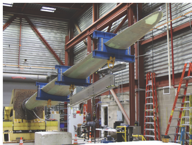
Fig. 1: 13 m thermoplastic blade at the test stand (c) Ryan Beach [7]
