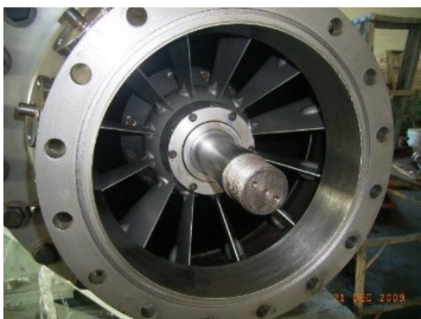
Fig. 1: Runner blade (top) and guide vane (bottom) of the small hydro propeller turbine [3]
