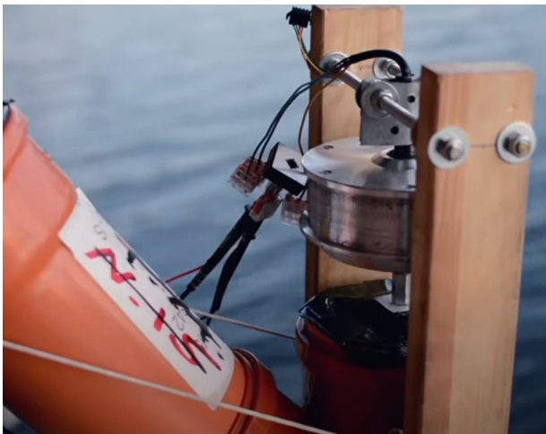
Fig. 4: Hoverboard wheel used as alternator [16]
