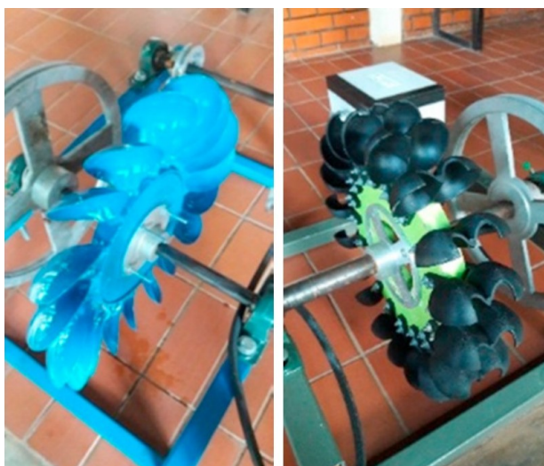
Fig. 2: Spoon-Based Turgo wheel (left) and 3D printed Pelton wheel (right) [15]
