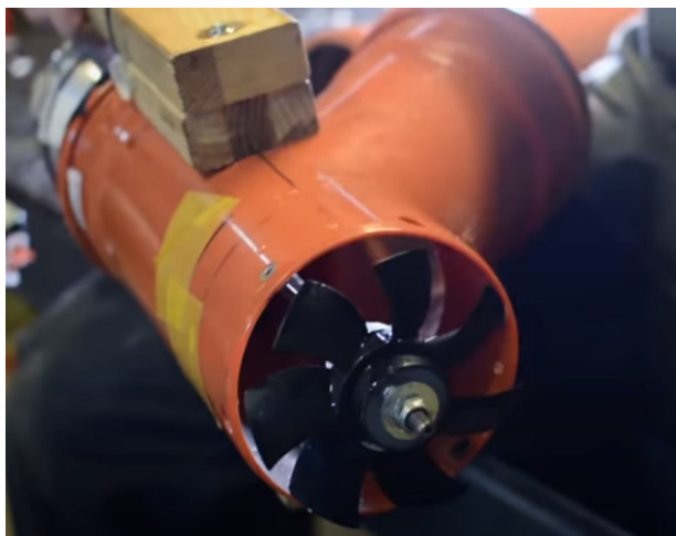
Fig. 3: Computer power supply PVC plastic fan as impeller [16]
