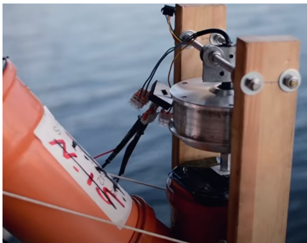
Fig. 4: Hoverboard wheel used as alternator [16]
