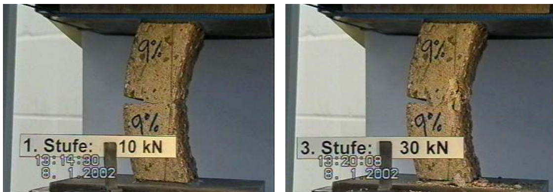
Figure 7. Old pipe sample, deformed 9 % at F = 10 / 30 \text{ kN} (= 15 / 45 % of the ultimate load)
